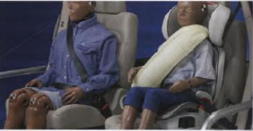
**Fig. 10.13** (*Left*) Advanced restraint (mesh webbing) for the pregnant occupant that can be added to a standard three-point belt for maximum fetal protection (Reproduced
