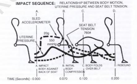
Fig. 10.8 Impact sequence (see test for details). Reproduced with permission from [90]
