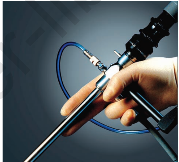
Figure 2.33 The single-puncture operating laparoscope for laser laparoscopy. The direct coupler containing the focusing lens is attached to the operative channel of the laparoscope
