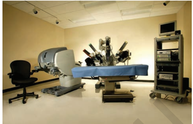
Figure 38.1 The complete robotic unit consists of a console, the robotic tower and the video cart. Courtesy of Intuitive Surgical
