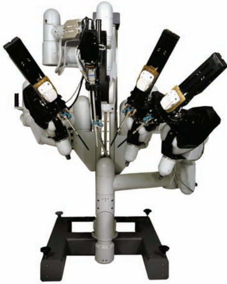
Figure 38.3 The robotic tower has three or four arms that hold instruments or the laparoscope. Courtesy of Intuitive Surgical
