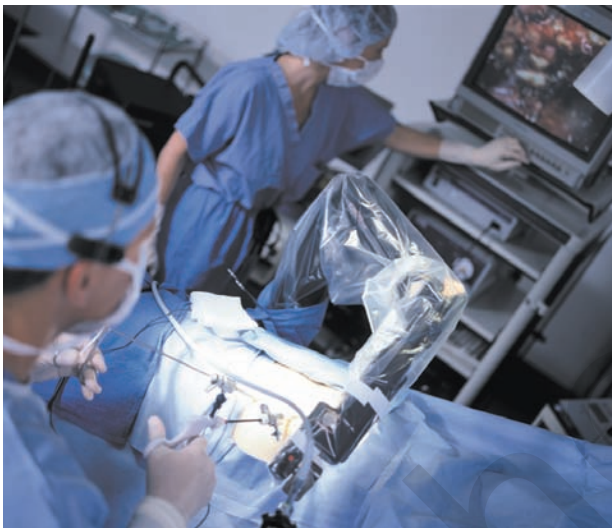
Figure 37.7 Aesop™ laparoscope holder (interface: voice)
