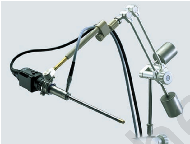
Figure 37.10 ImagTrack laparoscope holder (interface: finger)
