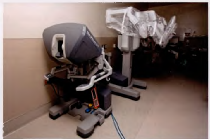
FIGURE 120-3 The robotic system is kept away from the operating table until trocars are in place and ready for docking. The surgeon's console is located away from the operating table. (© 2015 Intuitive Surgical, Inc. Reproduced with permission.)
