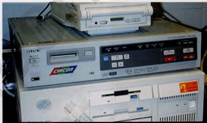
FIGURE 106-7 The digital printer permits permanent still picture records and slides to be produced from the operation.
