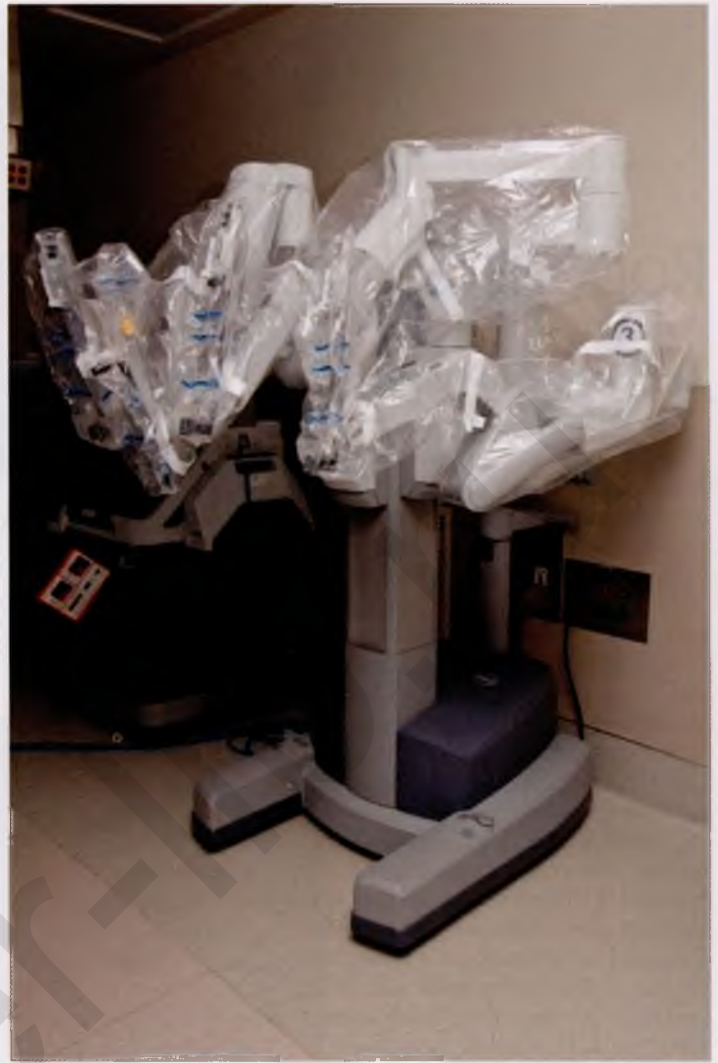
FIGURE 120-2 Da Vinci Si system with sterile plastic bags ready for surgery. (© 2015 Intuitive Surgical, Inc. Reproduced with permission.)
