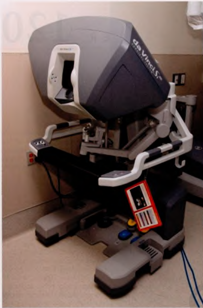
FIGURE 120-1 Surgeon's console of da Vinci Si system. (© 2015 Intuitive Surgical, Inc. Reproduced with permission.)
