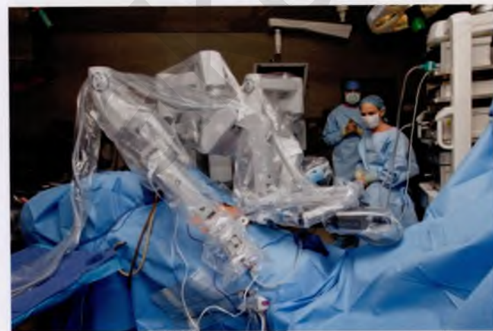
FIGURE 120-8 Docking of the da Vinci Si system is completed. The robotic column is right sidedocked. Once the robotic arms are docked to the patient trocars, the operating table cannot be moved unless the robotic arms are disengaged from the trocars. (© 2015 Intuitive Surgical, Inc. Reproduced with permission.)
