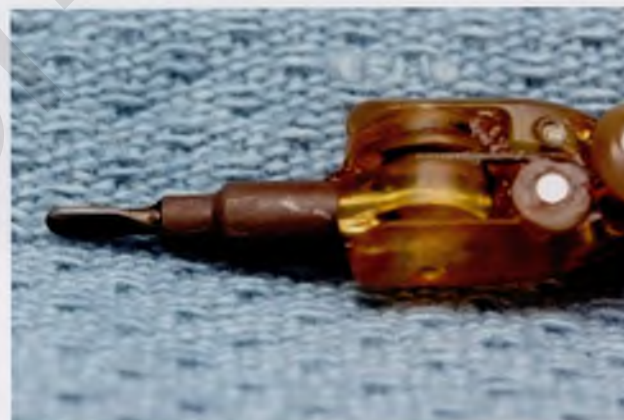
FIGURE 120-12 Monopolar spatula. It is a more precise coagulator than the monopolar scissors.
