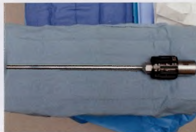
FIGURE 120-14 Robotic laparoscope. It is 12 mm in diameter and contains two fiberoptic channels to provide a three-dimensional image to the surgeon.
