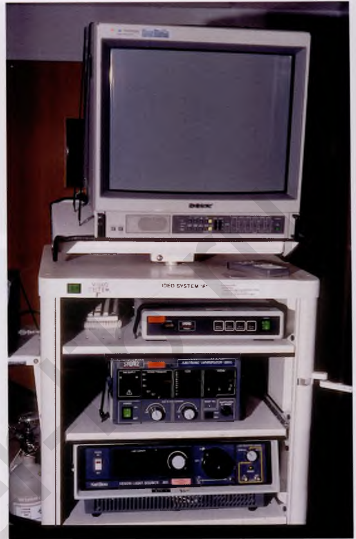
FIGURE 106-5 The large mobile instrument accessory cabinet contains a video monitor, a video control device, a fiberoptic light source, and a video recorder.
