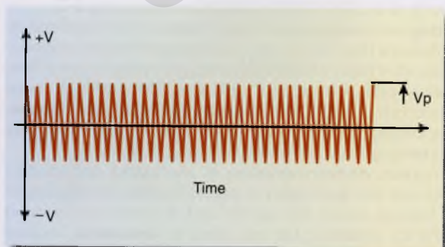
FIGURE 6-3 A typical oscilloscopic pattern for "cutting current." Note that the peak-to-peak voltage is relatively low and there is no modulation of amplitude. Current flow is high.
