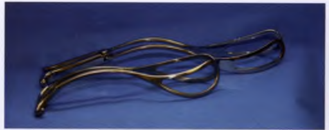
FIGURE 21-17 The Piper forceps (background) and Lafe-Piper forceps (foreground) are similar in shape but markedly different in length. The Piper forceps feature an English lock, in contrast to the pivot lock of the Lafe-Piper forceps. The pivot lock at the distal end of the handles makes the Lafe instrument divergent, that is, the branches never cross.
