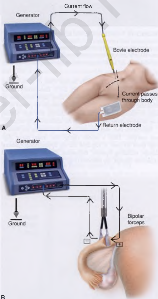
FIGURE 2-20 Circuits in electrosurgery. A. Monopolar electrosurgical circuit. B. Bipolar electrosurgical circuit. (Reproduced with permission from Balgobin S, Hamid CA, Hoffman BL: Intraoperative considerations. In Hoffman BL, Schorge JO, Bradshaw KD, et al (eds): Williams Gynecology , 3rd ed. New York, McGraw-Hill Education, 2016.)
