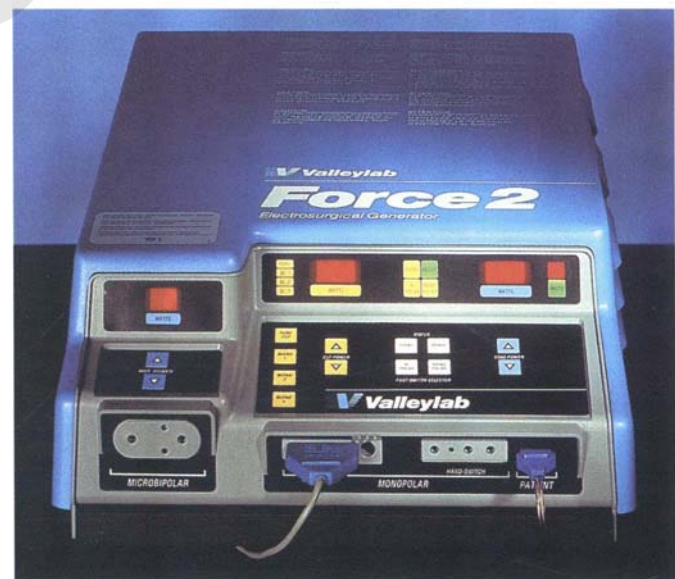
Fig. 7.47 A Valley Lab Force 2 electrodiathermy machine. These machines provide variable power for cutting and coagulation; the required power can be blended using a simple hand switch. The patient is "earthed" using an adhesive disposable jelly pad attached to the thigh. Use of the machine provides a high-quality cut resulting in minimal tissue damage through coagulation or thermal artifact. Hemostasis is easily and rapidly achieved. When the equipment is used in a modern colposcopy service it is important that there is no television interference.
