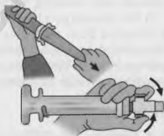
Fig. 19.8: Pulling out the plunger until arms snap out and rest on edges of the barrel
