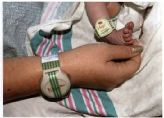
FIG 24-14 Mother and infant wear electronic bracelets as part of an infant security system. (Courtesy Shannon Perry, Phoenix, AZ.)
