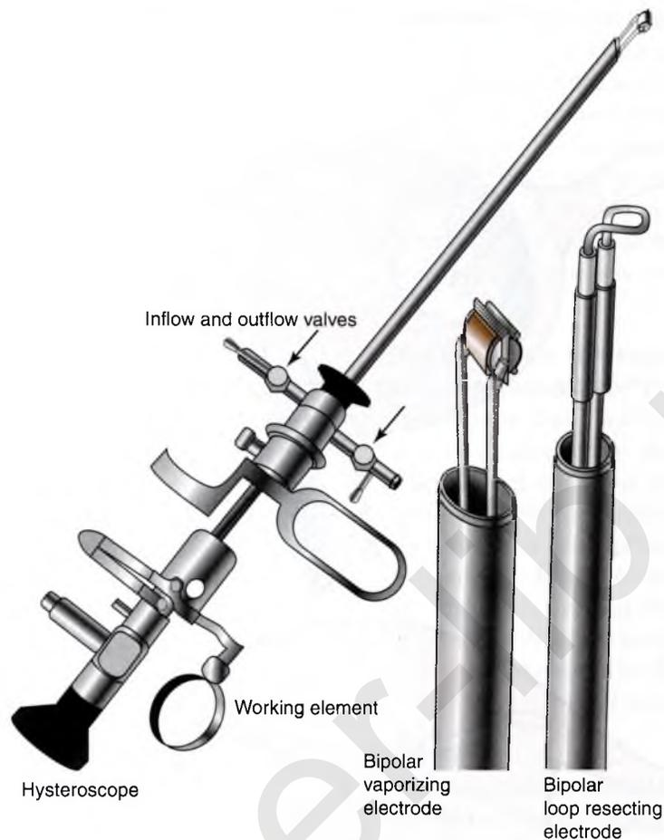
**FIGURE 1.6 Versapoint® Resectoscopic System (Gynecare, Inc.):** The Versapoint® vaporizing electrode measures 4 mm wide and 4 mm in diameter, while the wire loop electrode has a diameter of 2.5 mm. Either of these components attaches to the working element and sits within the 9-mm hysteroscopic sheath, which generally necessitates dilation of the cervix.
