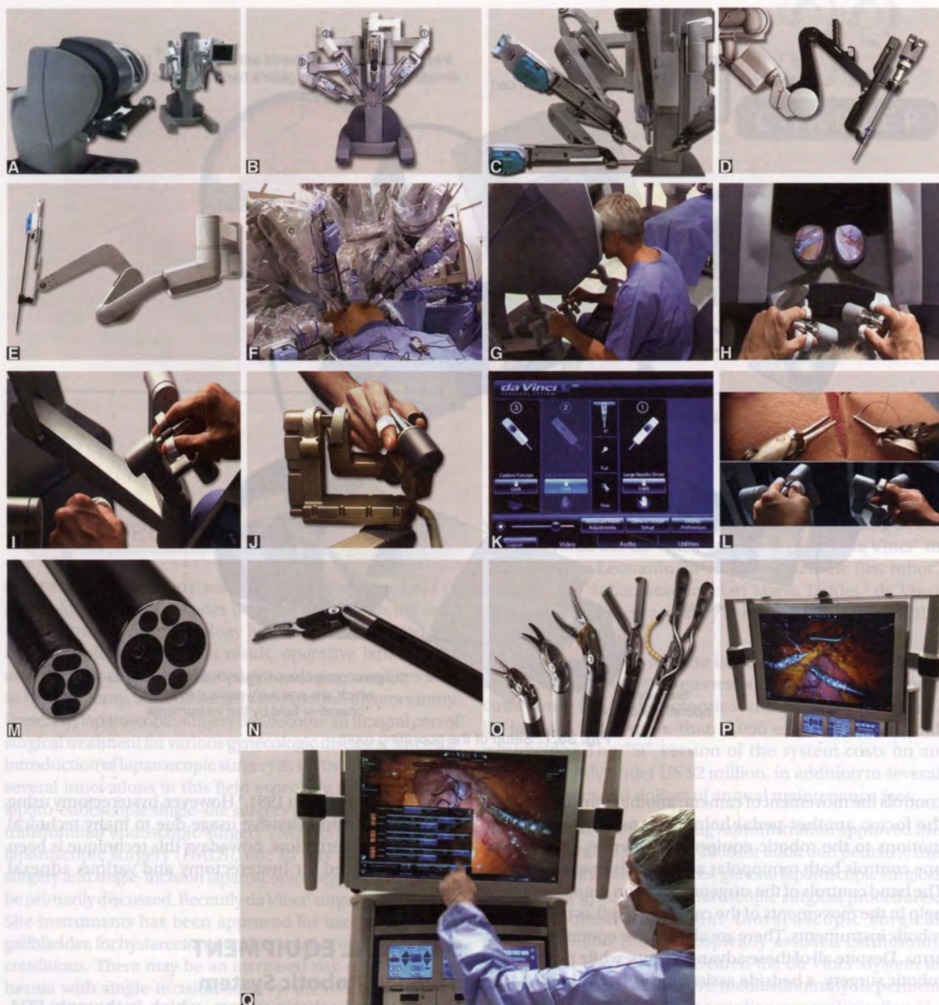
Figs 33.2A to Q: Robotic da Vinci® operating system. (A) da Vinci® robotic operating system along with the operating console where the surgeon sits; (B) Image of the robotic operating equipment cart from the front; (C) Magnified view showing the robotic operating equipments; (D) Camera arm; (E) Angled instrument arm; (F) Robotic operating equipment after being inserted into the patient's abdomen; (G) The operating console where the surgeon sits; (H) Cameras of the robotic system which help in providing magnified, 3-dimensional, high-definition view of the operating field; (I) Surgeon's hand controlling movement of robotic equipment; (J) Movement of surgeon's fingers controlling the movements of robotic equipment; (K) Operating surgeon's monitor screen for controlling the movement of various surgical instruments in the operative field; (L) Surgeon's fingers controlling the movements of the robotic equipment to stitch the abdominal incision; (M) A 12 mm and 8.5 mm endoscope; (N) EndoWrist® forceps; (O) Array of robotic equipment; (P) View of robotic surgery as visualized on the monitor of vision cart; (Q) An assistant surgeon changes the details of the monitor of the vision cart © 2015 Intuitive Surgical, Inc.
