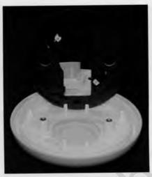
Figure 2-7. The tocographic transducer ('smart pulse'), which consists of two infrared sensors to detect superficial maternal vessel pulsations.
