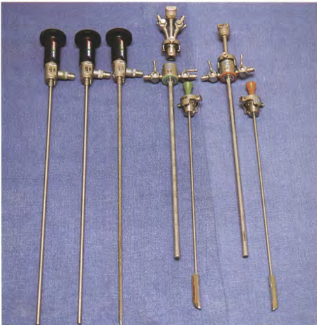
Figure 2.1 Basic cystoscopy set with telescopes 0°, 12° and 70°, sheath and bridge with biopsy channel, obturator, smaller sheath and bridge without biopsy channel and obturator
